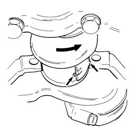
The upper bearing shell is installed by turning the crankcase the **opposite way to the normal direc-tion of rotation**, with the pin in the hole. Check that the pressed out heel in the bearing shell engages correctly in the cutout in the bearing seat. Remove the pin from the oil hole and install the cap with a new bearing shell.
